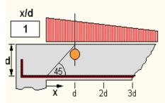
For continuous distributed loading, as indicated by the shear force diagram, the shear capacity is unchanged. Instead a reduction in shear force is generally effected by not considering the design shear force nearer than an effective depth, d from the face of a direct support.
